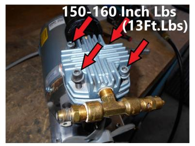
Tighten the cylinder bolts to 150-160 inch lbs. (Approx. 13 Ft. lbs.)
