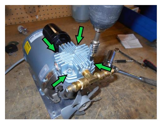
Remove the 4 head bolts and pull off the cylinder head and valves.
