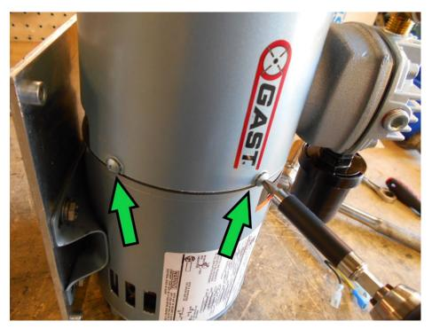
Remove the fan shroud by unscrewing the 4 fan shroud screws. Note that fan shroud screws have thread locking compound on them and may be difficult to remove. Using a heat gun to apply heat to the screws can assist in removal.
