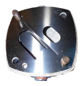
Place the exhaust valve onto the head. There is a small crease down the center of the valve, the raised side of this crease should be put towards the gasket. Once again note the alignment hole in the valve.
