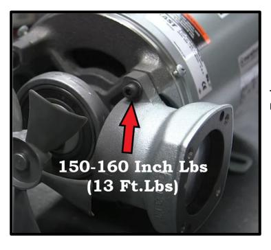
Tighten the cylinder bolts to 150-160 inch lbs. (Approx. 13 Ft. lbs.)
