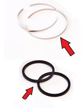
The piston rider ring is more difficult to install and will normally need to be held in place while reinstalling the cylinder over the piston. Fit the rider ring onto the piston and while holding it in place reinstall the cylinder over the piston seals while twisting the cylinder back and forth to get it to slide over the rider ring and down over the piston.
