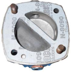
Put the head gasket onto the head ensuring the center cross piece lines up with the center divider in the head casting. Note the extra hole in the gasket that aligns with the alignment mark cast into the head.
