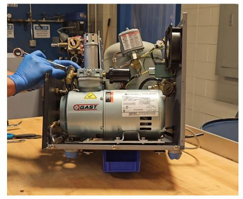
To allow for easier access, the compressor needs to be removed from the unit.
