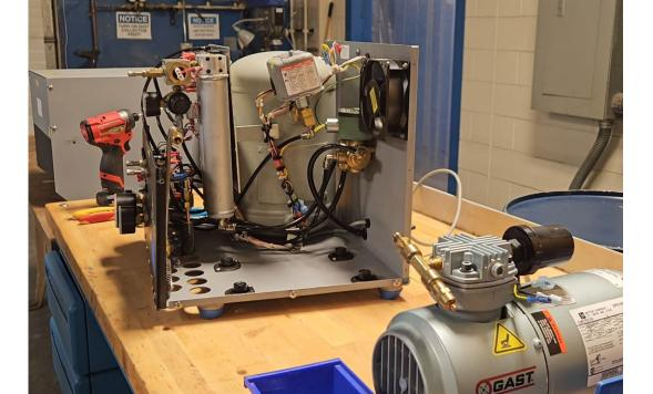
Remove the compressor from the unit to perform the rebuild.
