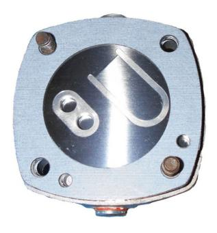
Install the cylinder gasket. This gasket has alignment marks but does not have any particular orientation and can be install in any direction. This concludes stacking all the valve components. Reattach the head to the cylinder paying special attention to the rotation of the head to the cylinder so that the intake filter and exhaust fittings are oriented correctly.
