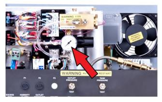
• If the backpressure setting requires adjustment, it can be adjusted with the regulator directly behind the gauge. Pull the knob straight out into the unlocked position and turn it clockwise to raise or counterclockwise to lower the backpressure setting. In some cases if the backpressure setting was right at or below 45 PSI and all other functions appear normal, increasing the backpressure closer to 50 PSI is the only corrective action required to clear the humidity alarm.
