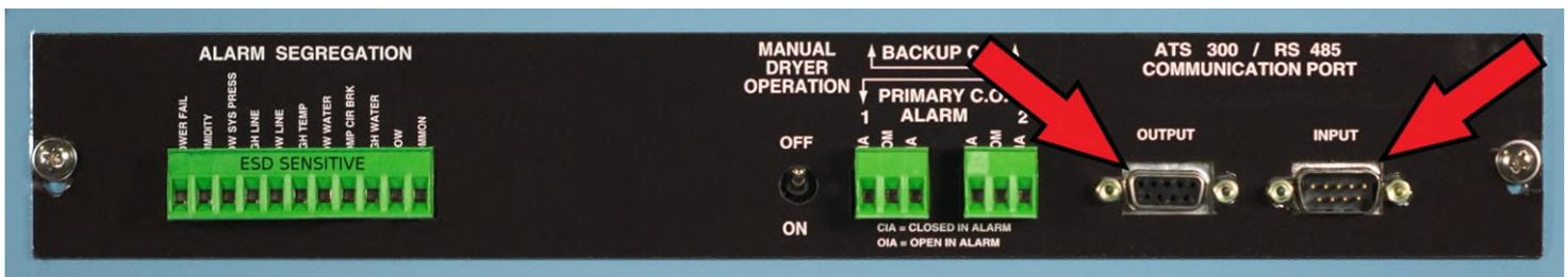
**Programming the ATS for Auto-rotation:** Before beginning to program the ATS300 ensure that each dryers serial address has already been programmed in the dryer setup menu (A1,A2...etc.) Refer to the dryer manual or dryer quick start guide for more information.
