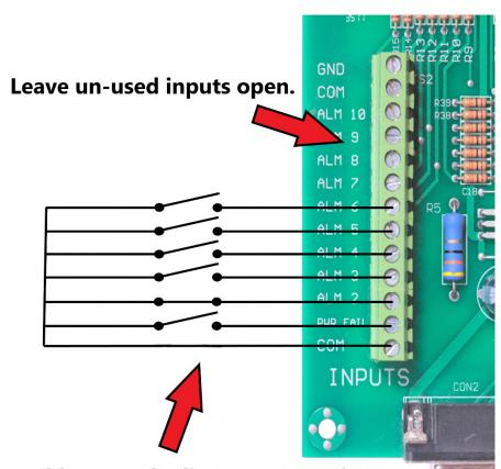
In this example diagram, ALM2 input has a closed connection between COM and ALM2 input terminal. ALM2 would be showing in alarm. All other inputs with open connections will show clear/no alarm.
