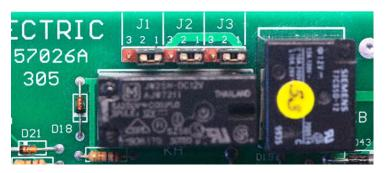
For "OPEN IN ALARM" configuration there are additional steps that must be taken to configure the interface board. There are 3 jumpers at the top of the board J1, J2 & J3 that must be moved from the factory default which connects pins 1&2 over to the setting for open in alarm by connecting pins 2&3 on each jumper.
