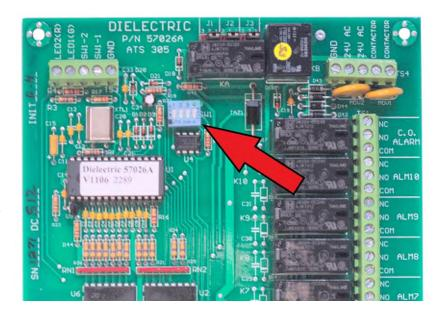
Set the dryer addressing with the DIP switch using the chart below.
