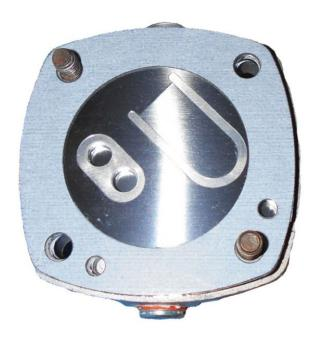
19. Install the cylinder gasket. This gasket has alignment marks but does not have any particular orientation and can be install in any direction. This concludes stacking all the valve components. Reattach the head to the cylinder paying special attention to the rotation of the head to the cylinder so that all of the intake and exhaust fittings line up correctly.
