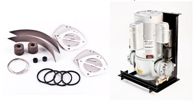
As a general recommendation it is advised to rebuild annually or every 2000 hours. The environmental conditions which the compressor is subjected to will have a great impact on service intervals. The compressor may require shorter or longer intervals between rebuilds depending on the condition of the parts observed when the compressor is disassembled.
