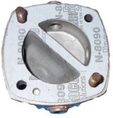
15. Put the head gasket onto the head ensuring the center cross piece lines up with the center divider in the head casting. Note the extra hole in the gasket that aligns with the alignment mark cast into the head.
