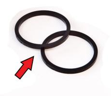
9. The piston rider ring is more difficult to install and will normally need to be held in place while reinstalling the cylinder over the piston. Fit the rider ring onto the piston and while holding it in place reinstall the cylinder over the piston seals while twisting the cylinder back and forth to get it to slide over the rider ring and down over the piston.
