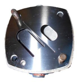
17. Install the vale plate on top of the exhaust valve. This is the thick metal plate included with the kit. This plate has two alignment marks so it must be observed that the intake and exhaust holes line up with the valves.
