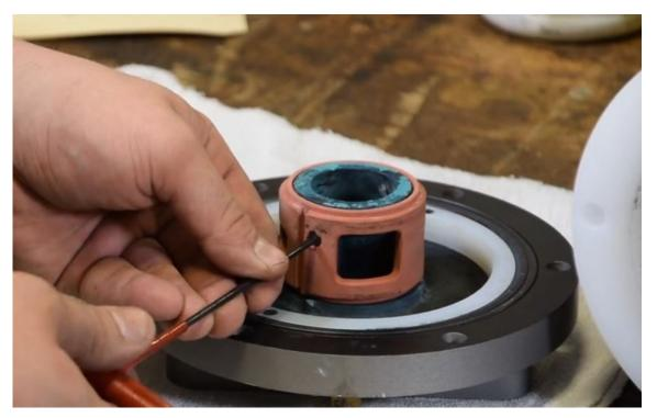
Using the 7/64<sup>"</sup> inch hex wrench remove the screw securing the portsleeve.
