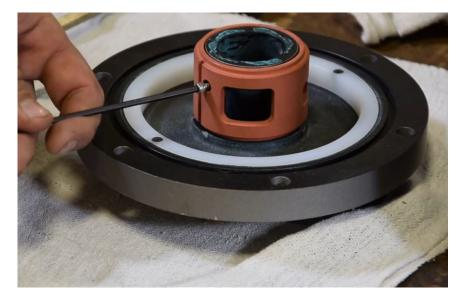
Reinstall the new port sleeve positioning screw.
