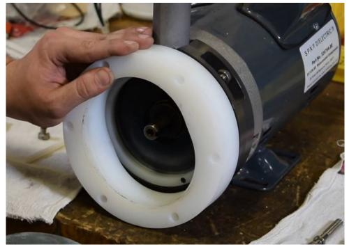
After the rotor is removed from the motor shaft, remove the housing by pulling it straight off of the housing base. There are two locating pins in the housing base and two corresponding holes in the housing for proper alignment during reassembly.
