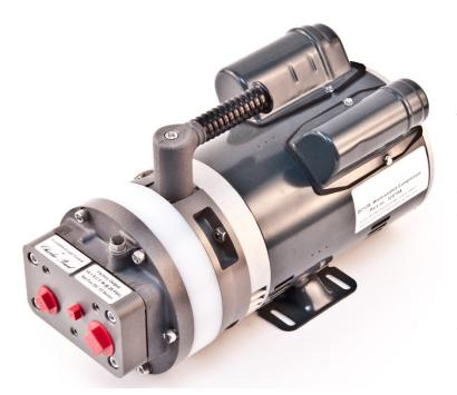
This guide will detail the necessary steps to rebuild the Dielectric water seal compressors using either the minor repair kit part number 47325 or the major repair kit part number 47328. Note that the two kits contain the same parts with the exception that the brass rotor is only included in the major repair kit. Rotor replacement is not normally required unless it is physically damaged or has been in service for many years.
