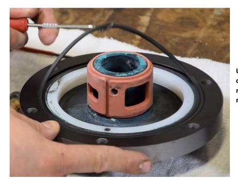
Using an O-ring pick, remove the large outer o-ring from the porthead. Lubricate the replacement O ring with silicone grease and reinstall into the groove on the porthead.
