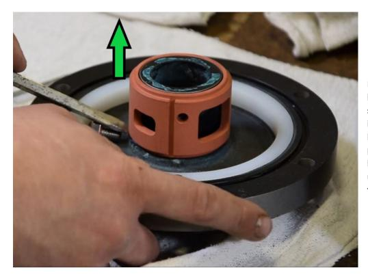
Pry the port sleeve off the porthead using the flat blade screwdriver. The rotor bolt included with the repair kit can be used as leverage to pry the port sleeve upward. Two flat blade screwdrivers can also be used on opposing sides to pry the port sleeve upward.
